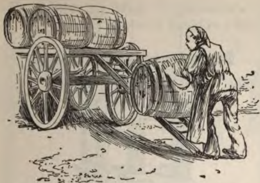
FIG. 101. A barrel too heavy to lift may be rolled up an inclined plane.
